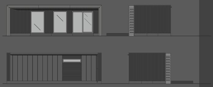
Elevation with full cladding across window openings.
